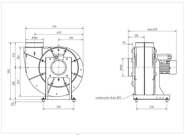
Gross weight of fan with motor approx. 15 kg, with  $\langle Ex \rangle$  approx. 20 kg
